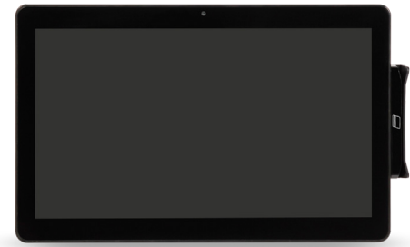
I-Series with MSR installed
